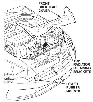
Install one washer from the kit on each side between the bulkhead and the radiator retaining brackets. Torque the bolts to 12 N·m (8.7 lb-ft).
