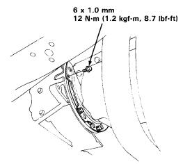
Install the control lever with the shift cable on the control shaft.
