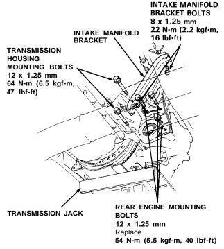
5. Install the transmission housing mounting bolts.
