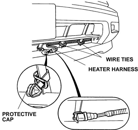
13. Reaching through the left front turn signal hole, secure the wire harness to the vehicle harness with one wire tie.
