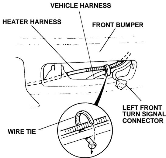
14. Secure the heater harness to the engine harness with six wire ties in the areas shown. Cut the excess off each wire tie.
