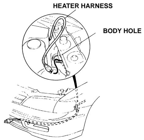
11. Attach the protective cap to the front grille, and plug the connector of the heater harness into the protective cap.
