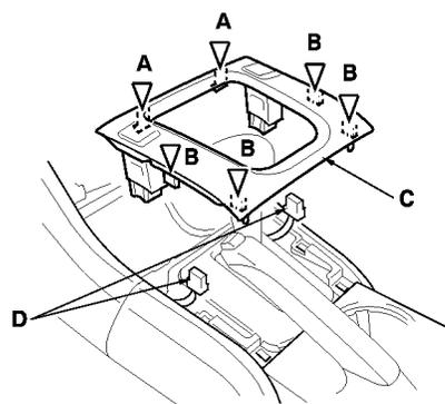
3. Pry up on the right of the console pocket (A) with a trim tool, and detach the clips, then remove the pocket.
