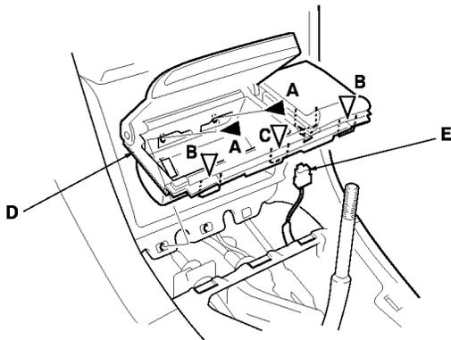
5. Detach the clips (A, B) by pulling the center console rear panel (C) up.
